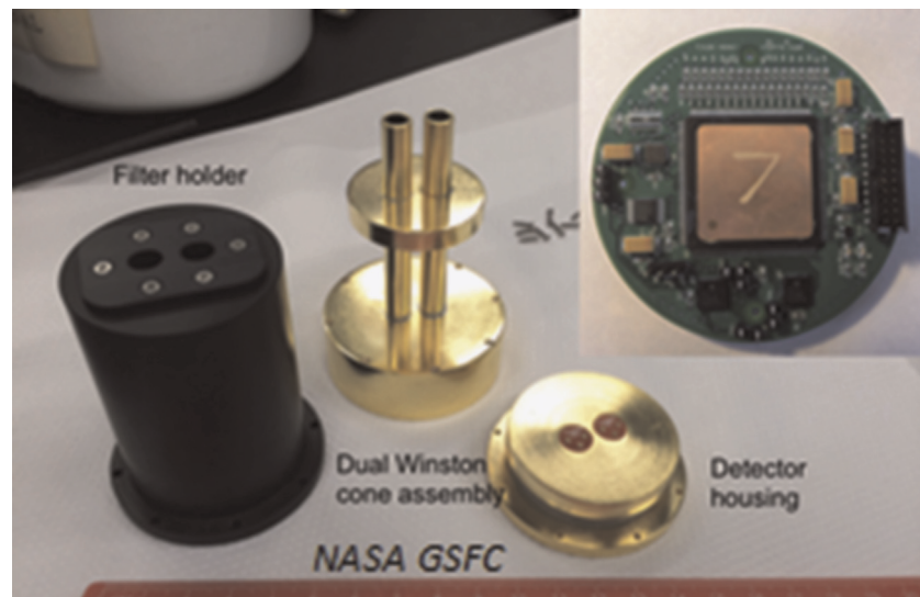
Fig. 5. NASA GSFC is testing early engineering models of the critical components the NFR. Dual Winston cone assembly and thermopile FEE readout (diameter ~70 mm) that uses a GSFC rad-hard mixed-signal ASIC (NASA GSFC).
